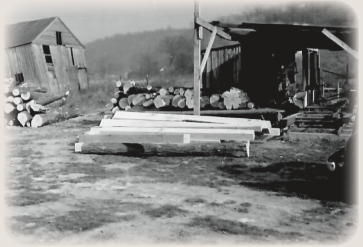
Black locust logs read to square up (left) for end posts and the finished posts (right). Rutherford Post Mill in Madison, Indiana, circa 1936. Photos by Roy C. Brundage.
