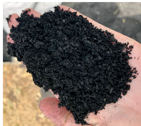
Figure 3. Image of the biochar applied on treated log landings. This particular biochar product was very finely textured, but some biochar can be very coarse, depending on its feedstock and how it was produced.
