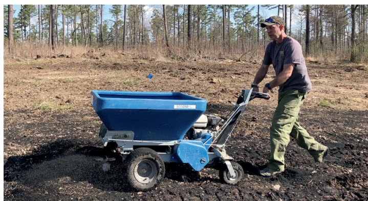
Figure 1. Chad Menke, former soil scientist and current fisheries biologist on the Hoosier National Forest, spreads biochar on a log landing to prep it for native plant seeding.
